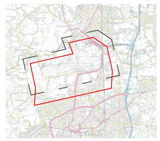
FIGURE 5.2 AIRPORTS COMMISSION 2030 DO-MINIMUM (BLACK) AND 2<sup>ND</sup> RUNWAY (RED) L<sub>AEQ,16HR</sub> 57 DB GROUND NOISE CONTOURS.
