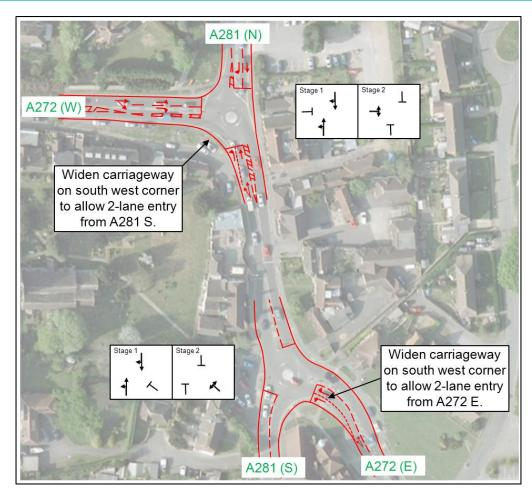
Figure 8: A272 / A281 Cowfold – Linked Traffic Signals, with 2-Lane Approaches
