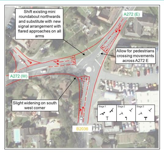
Figure 6: A272 / B2036 Ansty – 2-lane Approaches on Each Arm at Traffic Signals
