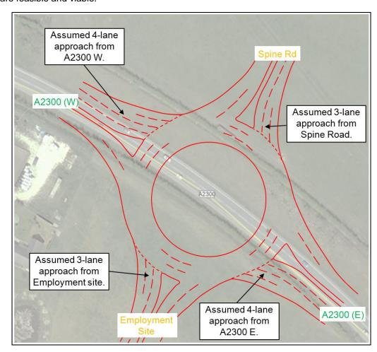
Figure 4: A2300 / Northern Arc Spine – Enlarged Roundabout
