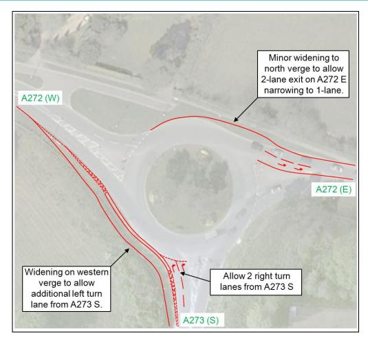
Figure 5: A272 / A273 Butlers Green – Widened Roundabout Approach and Exit
