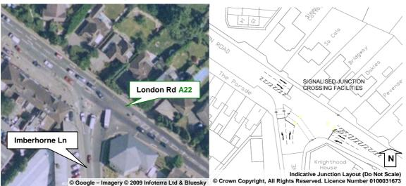
London Road has a total carriageway width of approximately 8m to the south of the junction. It consists of a single lane running in each direction which is flared on both arms in proximity to the junction to create dedicated straight and turning lanes. Similarly, the minor arm, Imberhorne Lane is flared in proximity to the junction to create dedicated right and left turning lanes.
