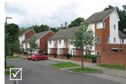
A mix of perpendicular and parallel parking may be possible but only if the street is well landscaped
