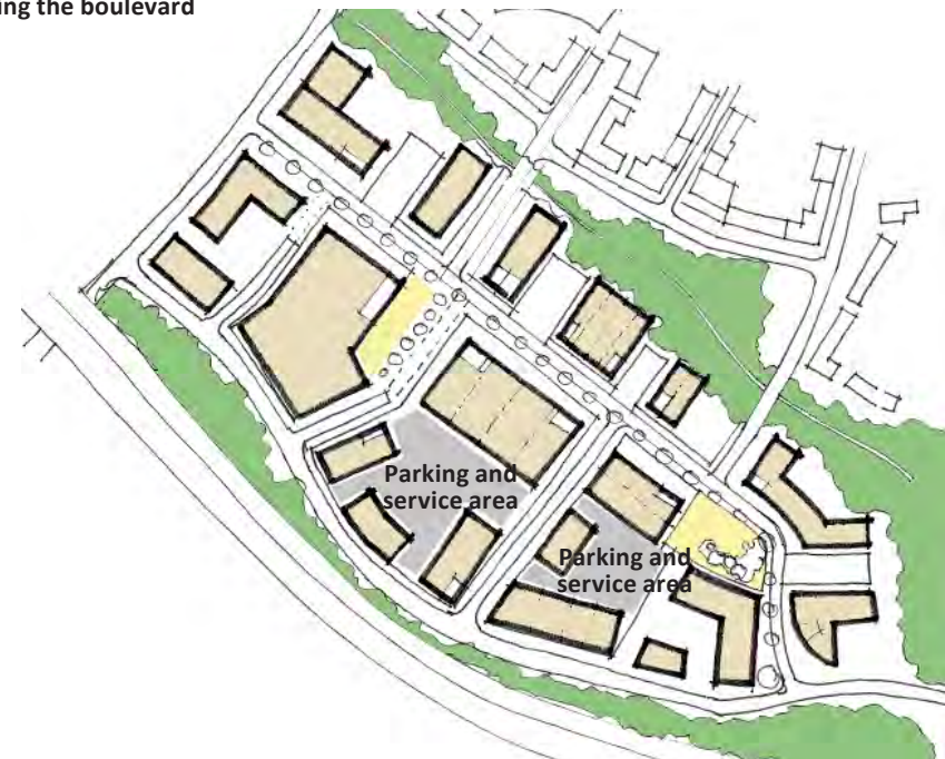
Figure 7C: Service yards and parking should be internalised within the perimeter block to reduce impact on the street environment
