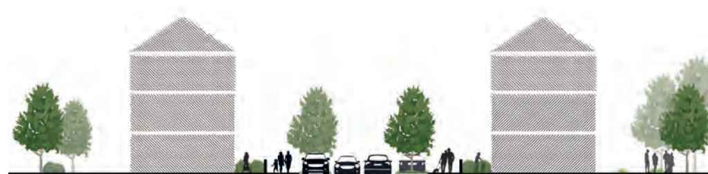
Figure 40: A good formal arrangement for a primary street that incorporates parallel parking with regular tree planting within kerb build outs reducing its impact on the street space (Section)
