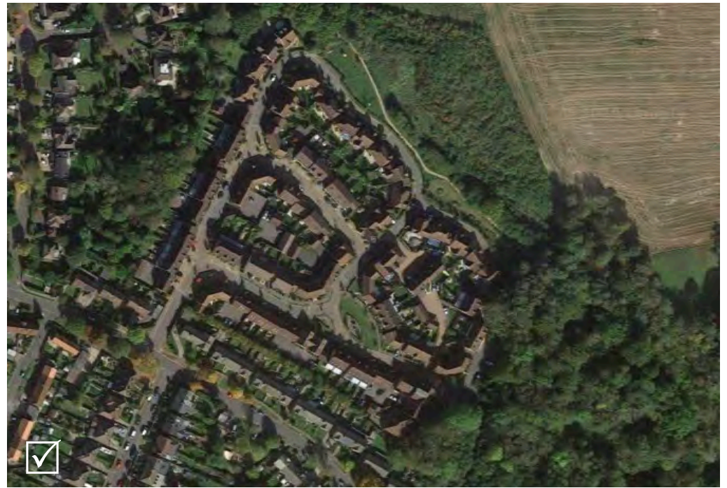
The layout of housing at Newton Road, Lindfield is arranged as a series of perimeter blocks (image courtesy of Google maps)
