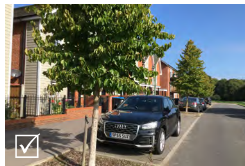
Parking is usually most unobtrusively accommodated on-street as parallel spaces softened and defined by tree planting
