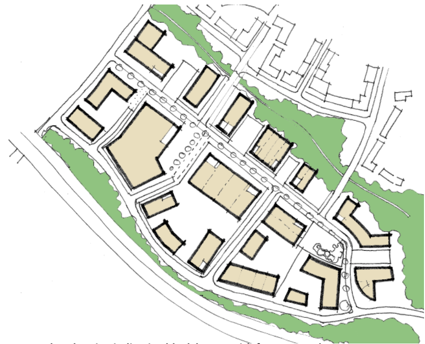
Figure 7B: Layout plan showing indicative block layout with frontage and entrances overlooking the boulevard
