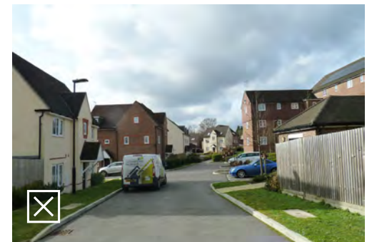
The use of close panel timber fencing to define the highway boundary is unacceptable
