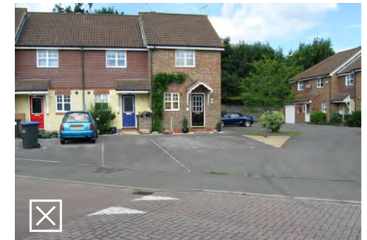
A set-back frontage generates weak street enclosure particularly when it is not compensated by trees/ soft landscaping and is instead dominated by parking and hard-standing
