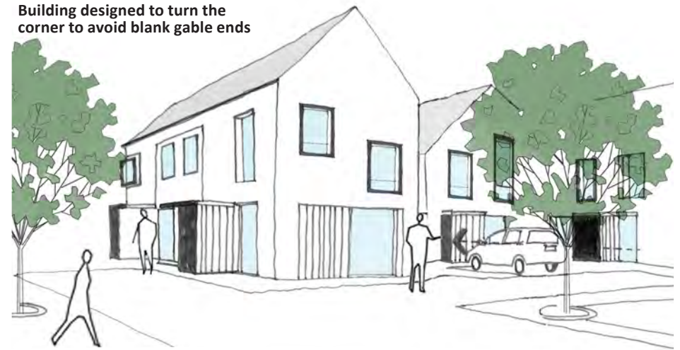
Figure 6I: Gable ends which incorporate windows provide overlooking
