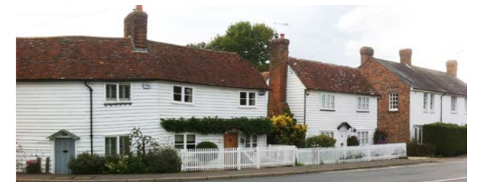
This streetscene in a High Weald village shows the characteristic grouping of a mixture of terraces, detached cottages, and semi-detached dwellings, each different in detail, but with common scale, building line, fenestration pattern, roof orientation and articulation with chimneystacks
