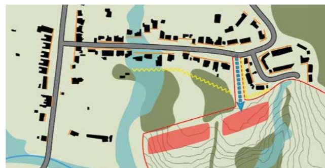
Site analysis diagram examining potential of site with regard to topography, watercourses, woodland and hedgerow, access, routes and adjacent street patterns and building grain
