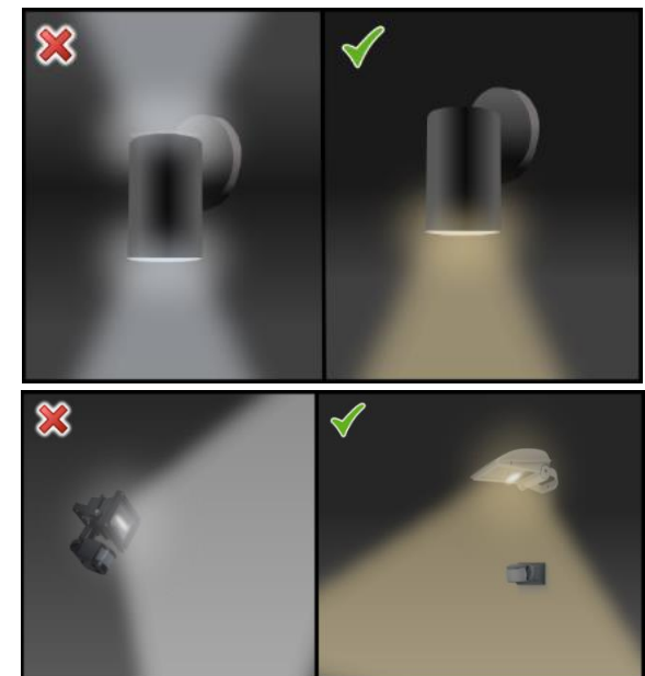
Fig 8: external lighting fittings – right hand images show directional, shielded light creating less upward skyglow.
