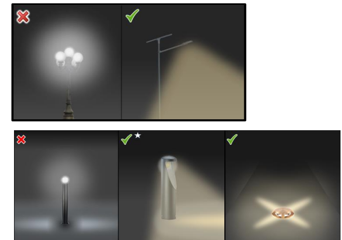
Fig 11: street lighting and bollard lighting - directional, shielded light installations create less upward skyglow.
