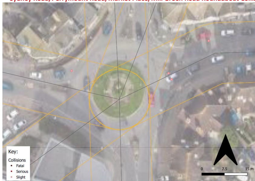
Figure 42. Sydney Road/Perrymount Road/Market Place/Mill Green Road Roundabout Collision Locations
