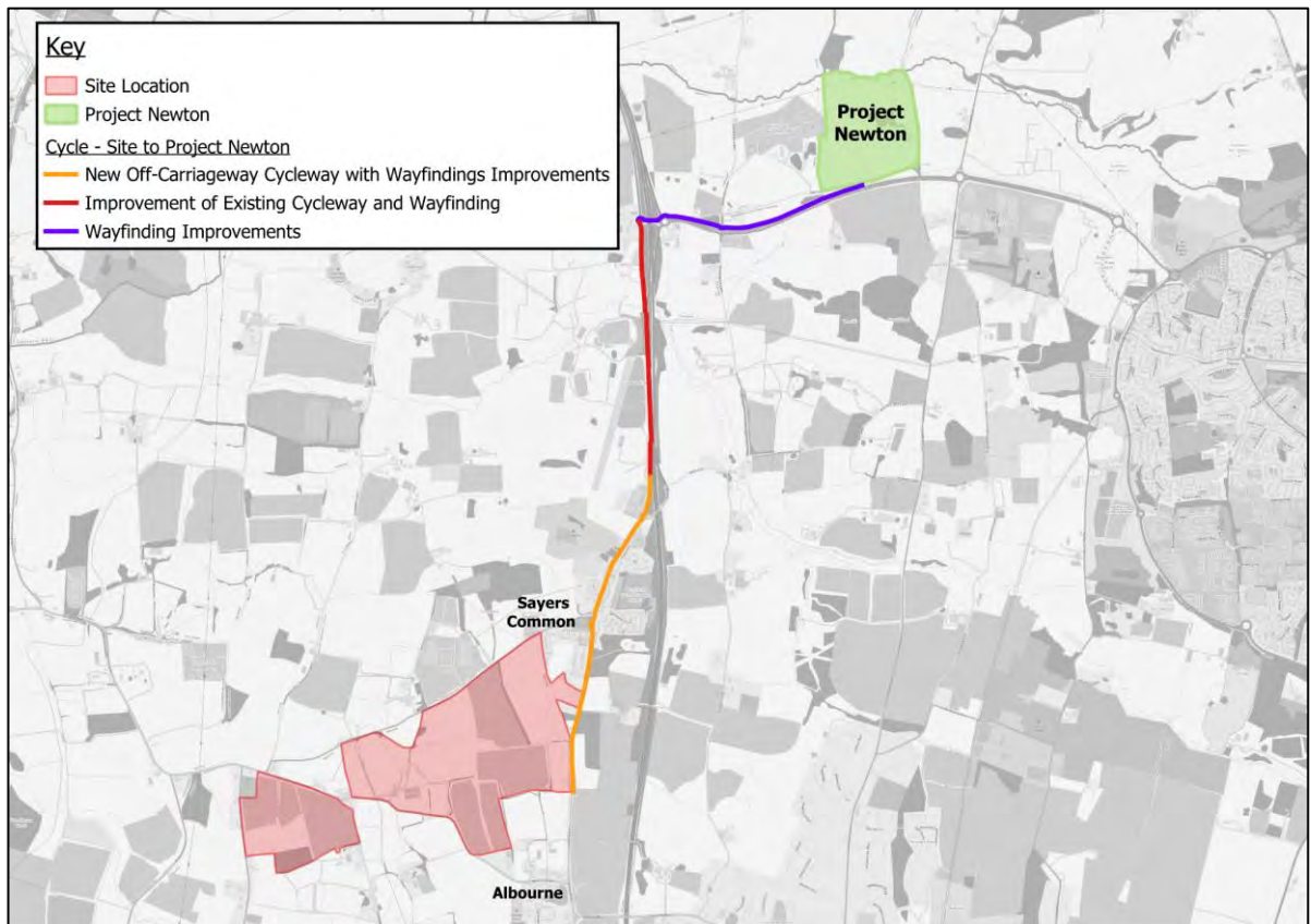
Figure 3.4 Potential Off-site Cycle Improvements – Route 2
