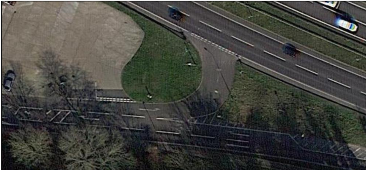
Figure 130. Northbound On-slip Layout – Give-way Merge
